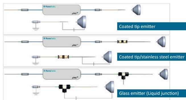
Figure 1: Grounded electrospray ionisation interfaces
