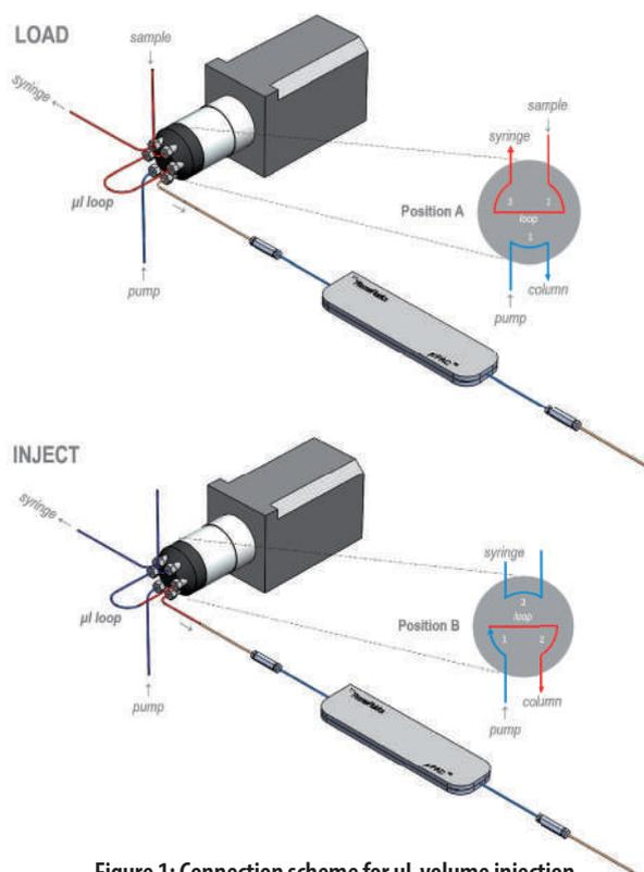
Figure 1: Connection scheme for  $\mu$ L volume injection
