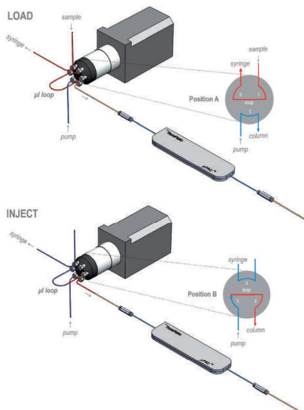
Figure 1: Connection scheme for µL volume injection
