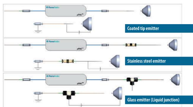
Figure 2: Overview of grounded electrospray ionisation interfaces
